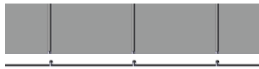
Standing Seam Metal Roof
